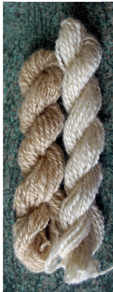
Sample skeins, left spun from greasy fleece, and right, spun from scoured fleece
