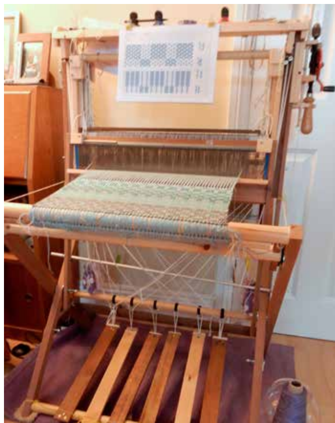
Home-made four-shaft loom with summer and winter towels
