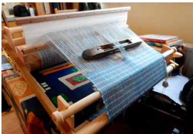
Jacket fabric on home-made rigid heddle loom
