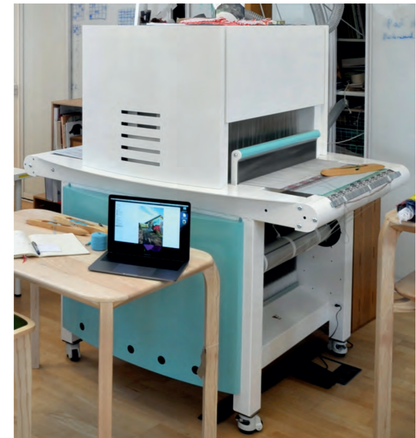
The TC2 electrical digital Jacquard loom
