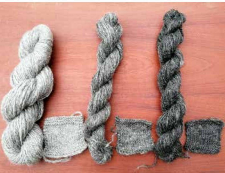
Semi-worsted plus alpaca skeins From left: Semi-worsted (Spinning Style, sample 2), mid grey plus black alpaca (Blending, sample 3); dark grey plus black alpaca (Blending, sample 2) Photo: Sonya Hammond
