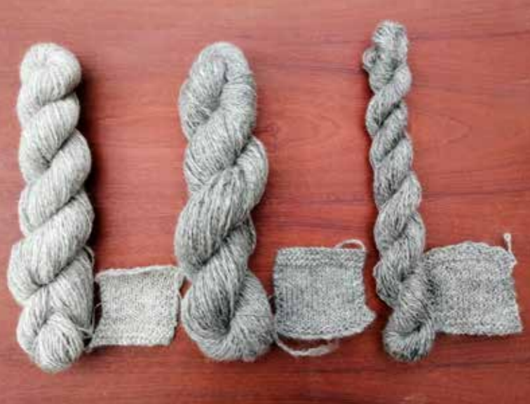
Spinning style skeins From left: Sample 1, semi-woollen; sample 2, semi-worsted; sample 3, fully worsted Photo: Sonya Hammond
