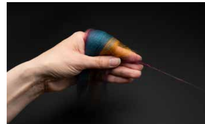
fig. 6 Joining a new section of fibre
